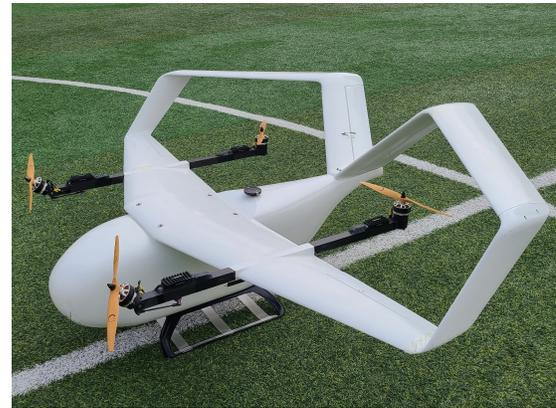
**Fig. 21:** Scale model of box-wing aircraft during flight test
